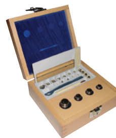
Set of fine increment masses
